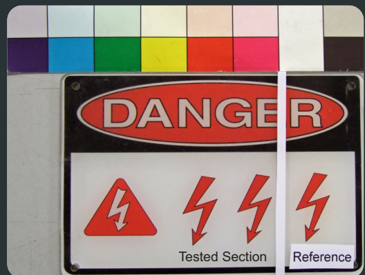
Test sample having undergone accelerated testing
